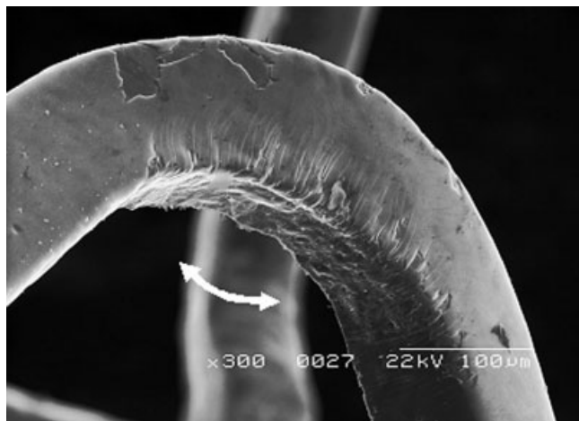
Figure 3. SEM microstructure of a-C:H coated stent after expansion. The film of thickness about 1\ \mu\text{m} was coated by an ion plating method using benzene. The arrow shows the expansion direction. Array of the cracks perpendicular to the direction of the stress were observed in the tensile side, while spallations of the coating were observed in opposite side where compressive stress was evolved during expansion.
