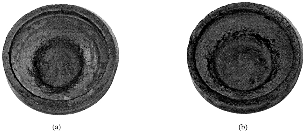
Fig. 5. Morphologies of the used cathodes eroded with both the permanent magnet and the yoke. The source magnet current was oscillated in the range of (a) 0.0~1.0 A and (b) 0.0~1.5 A
